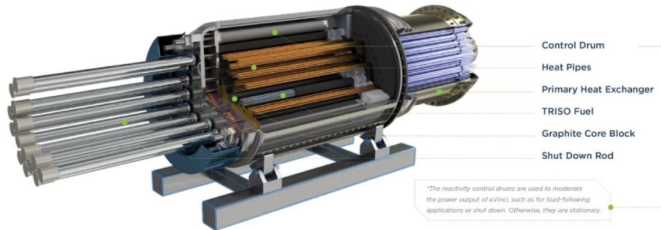
Figure 18 eVinci reactor core cutout showing the main components [2]
