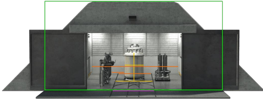
Figure 37 Rendering of the BANR reactor bunker [57] with an overlay of lines used in the estimation of the bay dimensions
