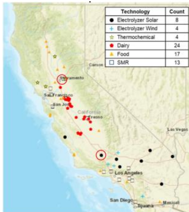
Figure 11 Suggested locations for hydrogen production facilities of different technologies by 2030 in the low hydrogen demand scenario of [10]. Electrolyzer wind/solar refer to (centralized) electrolysis with wind/solar energy, thermochemical refers to facilities producing hydrogen from biomass from forests and agricultural residue, dairy facilities make hydrogen from anaerobic dairy digesters, food refers to hydrogen production from the residential waste stream, and SMR refers to steam methane reforming
