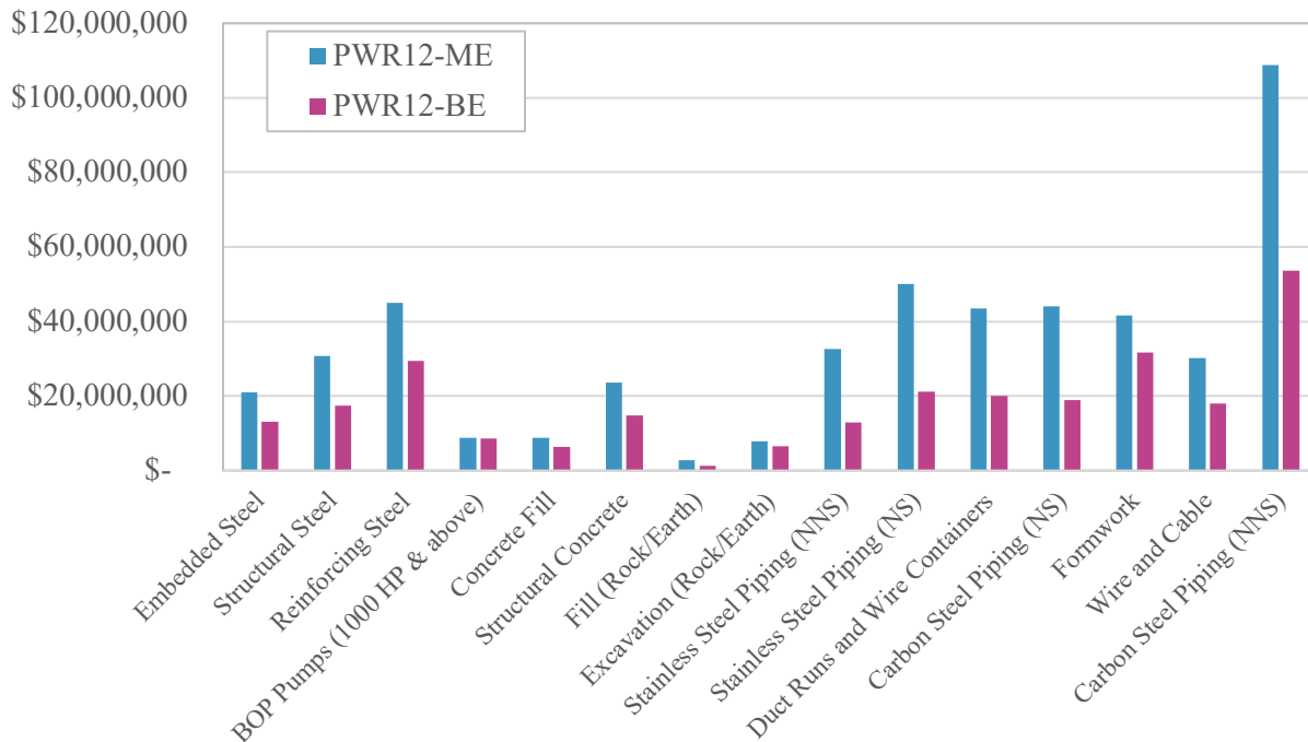
Figure II.3 PWR12 material cost from EEDB for the Better Experience and Median Experience cases by material type (1987 USD).
