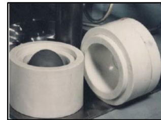
Figure 4-10 Completed spherical compact and furnace mold. Taken from [19]
