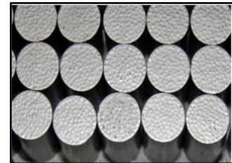
Figure 4-8 Complete cylindrical compact. Taken from [18]
