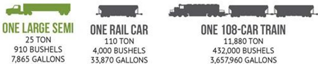
Fig. 6.2. Relative Capacity of Different Modes of Shipping Bulk Commodities [Iowa Department of Transportation 2019]
