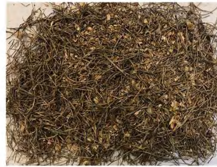
Air classified "Light" dirty fraction with fan speed of 3.8 m/s air velocity.
