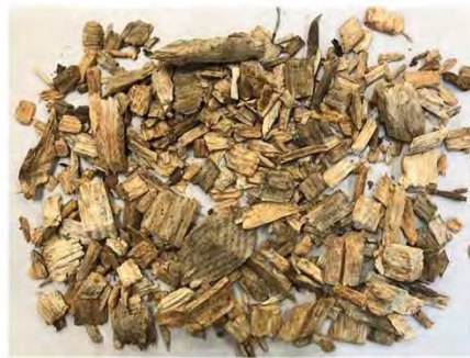
Air classified "Heavy" clean fraction with fan speed of 3.8 m/s air velocity.
