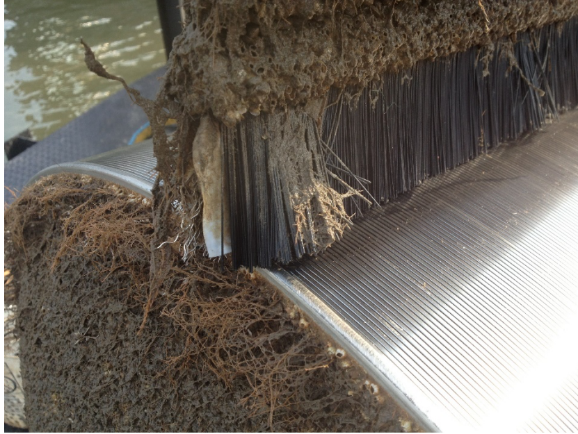
Figure 8. ISI mechanical brush-cleaned screen operating in Hudson River (Appendix A – Intake Screens, Inc. Report).
