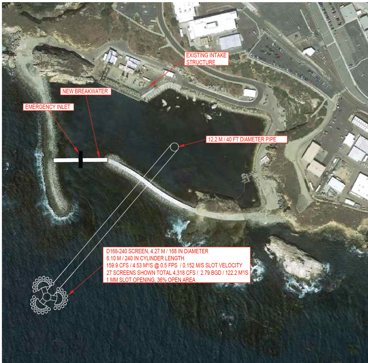
Figure 11. Aerial view of DCNPP with extended breakwater to isolate lagoon, emergency inlet structure, tunnel extending offshore, and wedgewire screen array for Option 1 (Appendix A – Intake Screens, Inc. Report).
